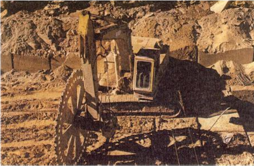
FIGURE 2.3 SANDSTONE CUTTING EQUIPMENT
